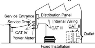
Using a measurement instrument in an environment designated with a higher-numbered category than that for which the instrument is rated could result in a severe accident, and must be carefully avoided.
