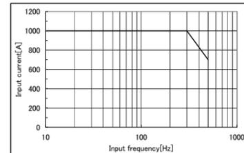
Figure 1. Permissible current to frequency
